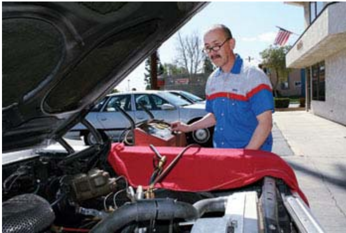
ASE Certified Technician Benjamin "Benny" Balderrama of Lynn's Auto Air uses a Robinair R12 machine to evacuate and recharge the custom air-conditioning system in a classic Chevy Malibu.
